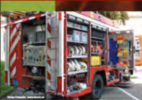
6 Below: The apparatus with compact station in the rear and compact design for maneuverability and access of curbside streets.
